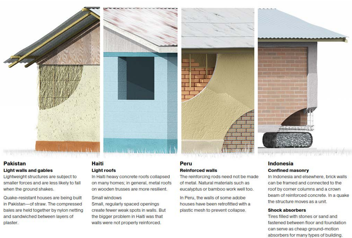
Figure 6.38. Alternative earthquake-resistant construction techniques proposed by researchers
