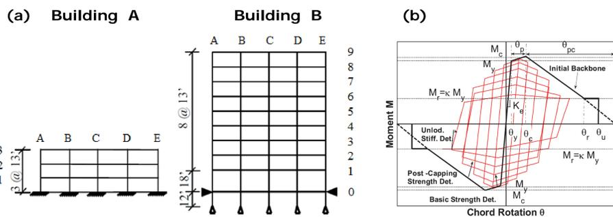
Figure 2: a) SAC steel frames (FEMA 2000); b) Hysteretic model of plastic hinges (Lignos et. al., 2011).
