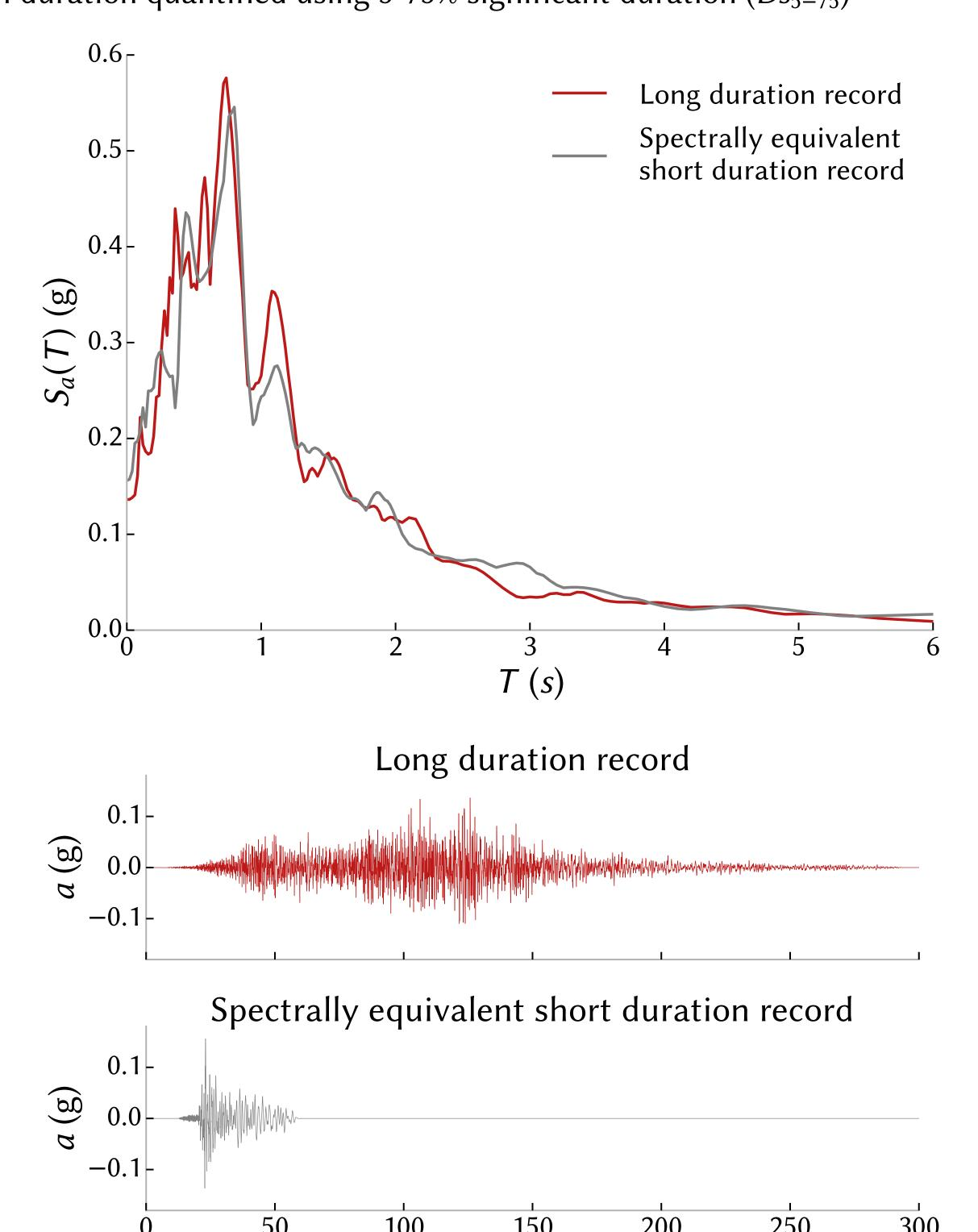
▶ Each ground motion was used to estimate a five-story steel moment frame's collapse capacity: the lowest  $S_a(T_1)$  value it needs to be scaled to, to cause structural collapse
