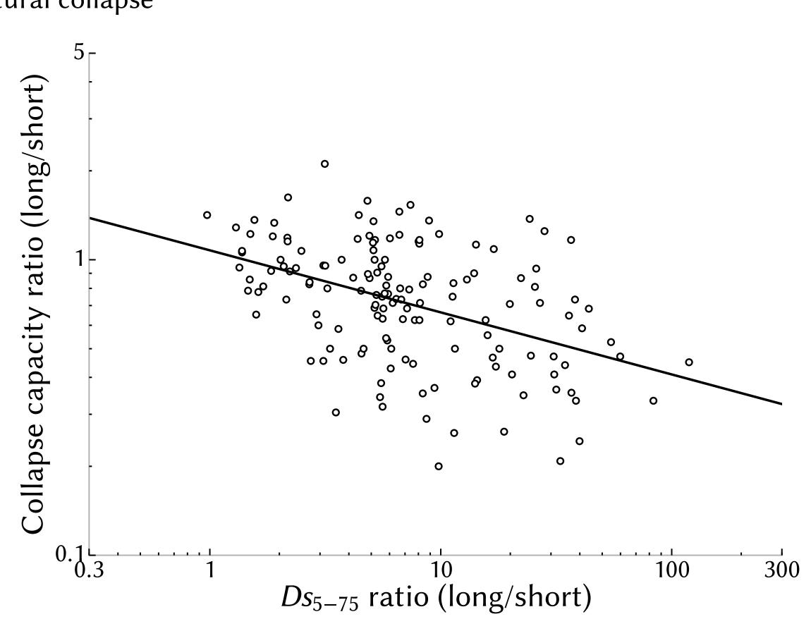
Results help quantify the influence of ground motion duration on structural collapse capacity while controlling for the effect of response spectral shape
