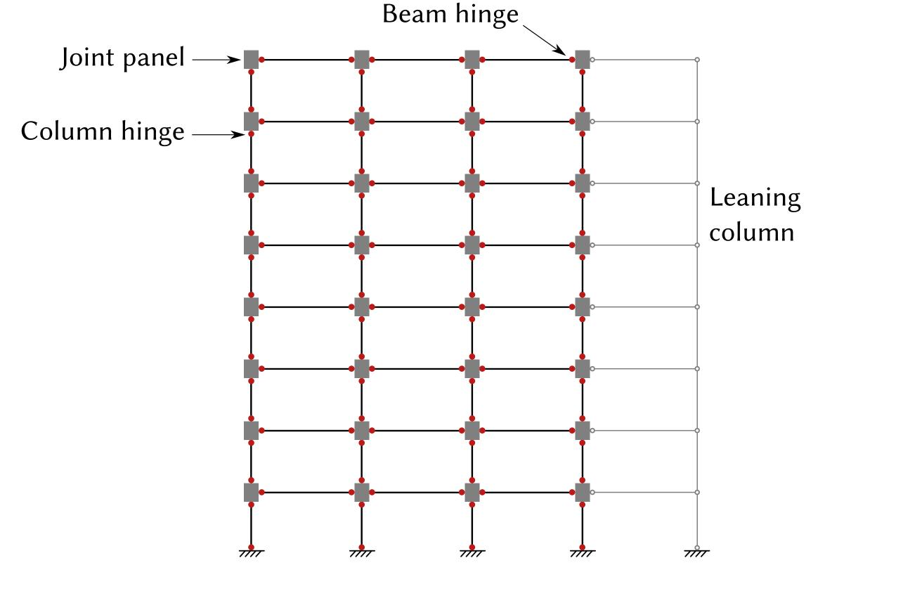
► Model incorporates the strength and stiffness deterioration of structural components and destabilizing  $P - \Delta$  effects: both characteristics required to capture the effect of duration
