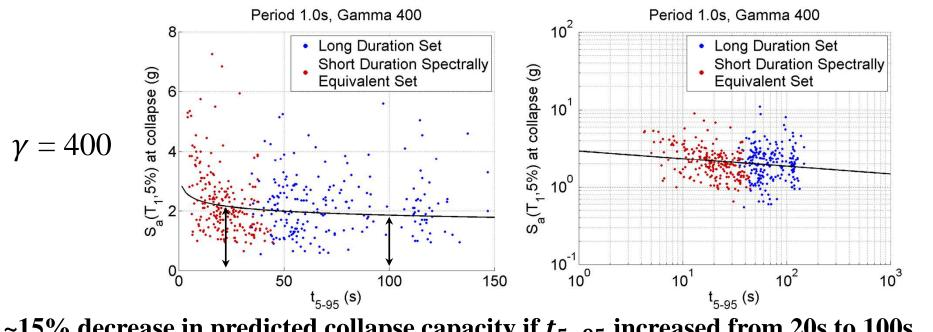
~15% decrease in predicted collapse capacity if  $t_{5-95}$  increased from 20s to 100s
