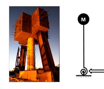
Concrete column tested by PEER and NEES at UC San Diego Modeled as an SDOF system
