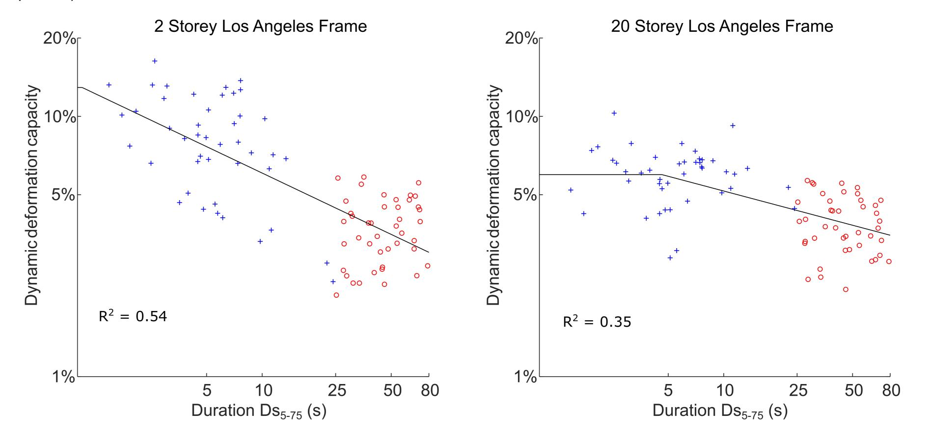
$\blacktriangleright$  The variation in dynamic deformation capacity with duration is investigated by plotting deformation capacity against  $D_{S_{5-75}}$ . Considering that deformation capacity is not expected to increase indefinitely under extremely short duration ground motions, a bilinear regression model is fit to the data points on logarithmic scales.
