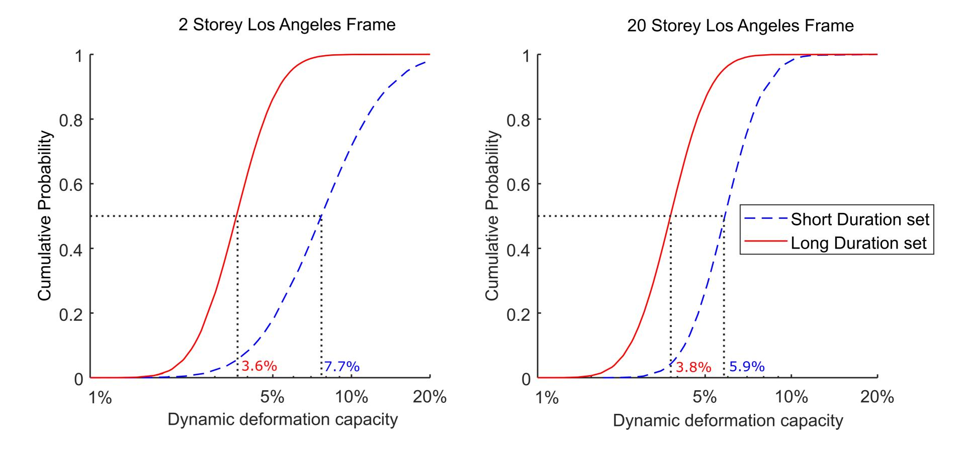
The median dynamic deformation capacity of the two-storey Los Angeles frame is estimated to be 3.6% and 7.7% using the long duration and
