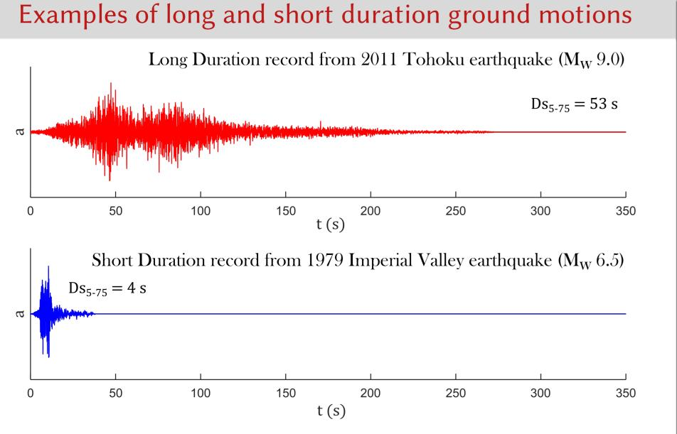
▶ 5-75% Significant durations  $(D_{S_{5-75}})$  of ground motion records from the 2011 Tohoku ( $M_W$  9.0) earthquake were as long as 80 s.
