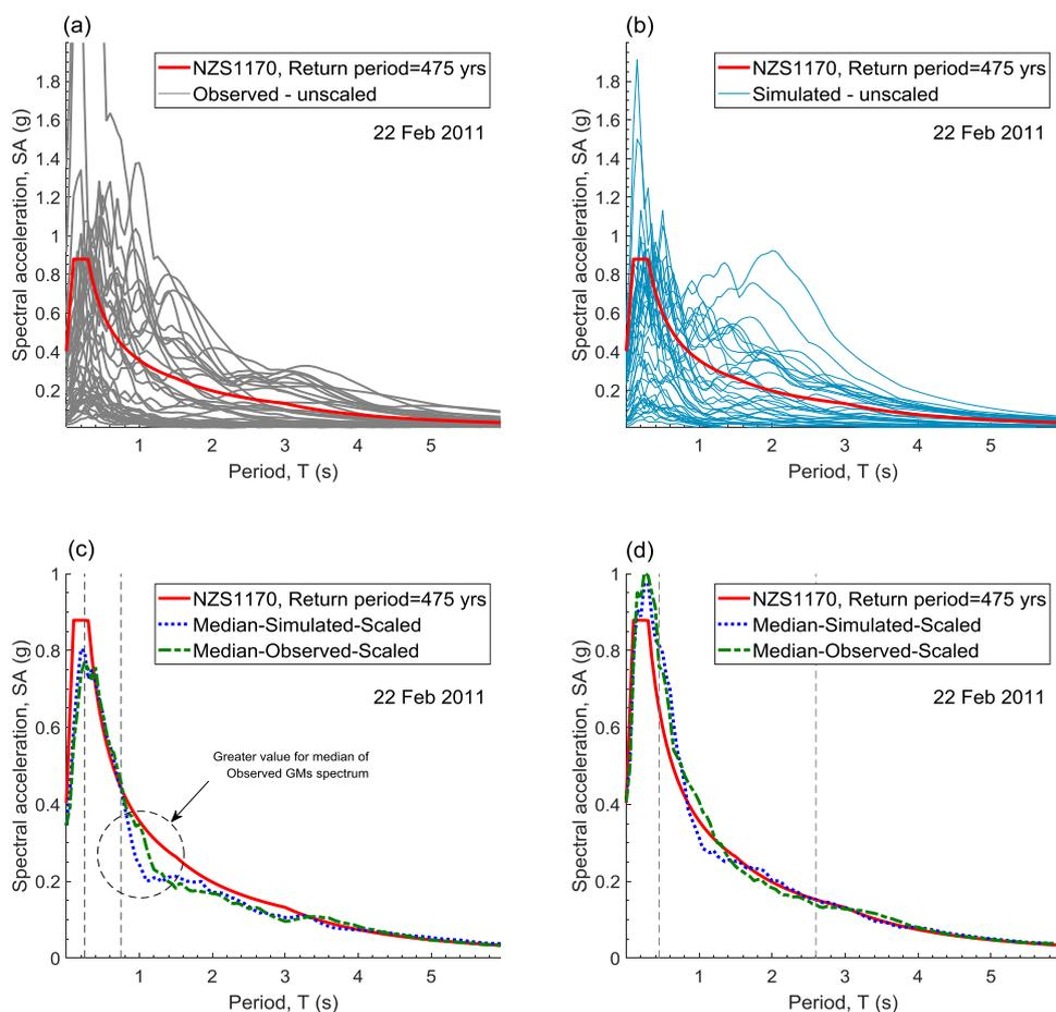
Figure 2: (a-b) Unscaled response spectra for the 40 observed and simulated GMs; (c-d) median of scaled response spectra for Building A and B.
