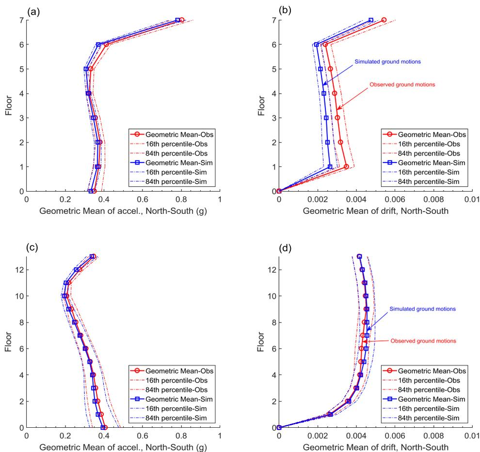
Figure 4: Geometric mean and percentiles of bootstrapped samples (a-b) Building A peak floor acceleration (PFA) and inter-storey drift ratio (IDR); (c-d) Building B PFA and IDR.
