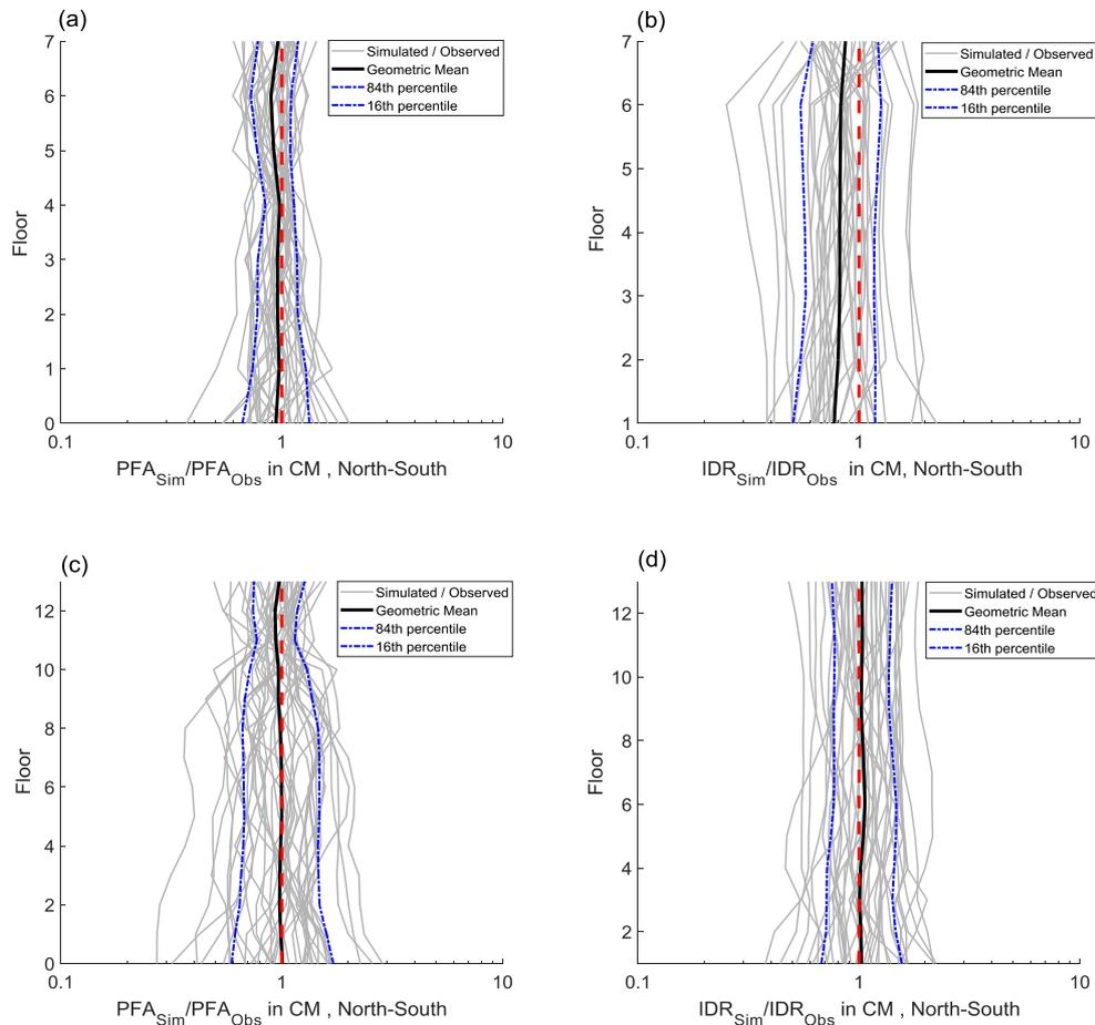
Figure 3: The ratios, geometric mean, and percentiles of simulated to observed responses (a) Building A peak floor acceleration (PFA); (b) Building A inter-storey drift (IDR); (c) Building B PFA; (d) Building B IDR.
